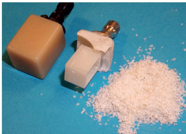
Fig. 4 Waste RBC particulates from CAD/CAM applications
